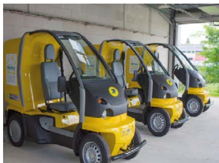
Fig. 1: MobyPost vehicles – First fleet of FCV in France (FC powertrain integrated @ FCLAB / UBFC)
